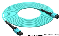
MPO-MPO Low Smoke Halogen Free Strain Multimode 10 Gigabit 24 pole OM3 Standard length: 10.00m Return loss: <math>15\text{dB}</math>
